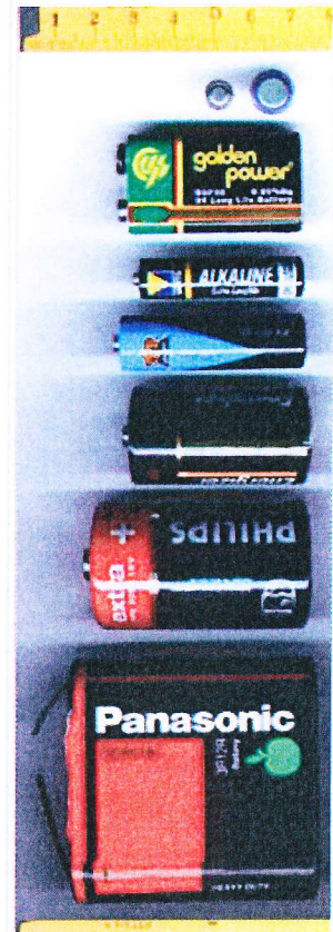
From top to bottom: SR41/AG3, SR44/AG13 (button cells), a 9-volt PP3 battery, an AAA cell, an AA cell, a C cell, a D Cell, and a large 3R12. (Ruler in centimeters.)
